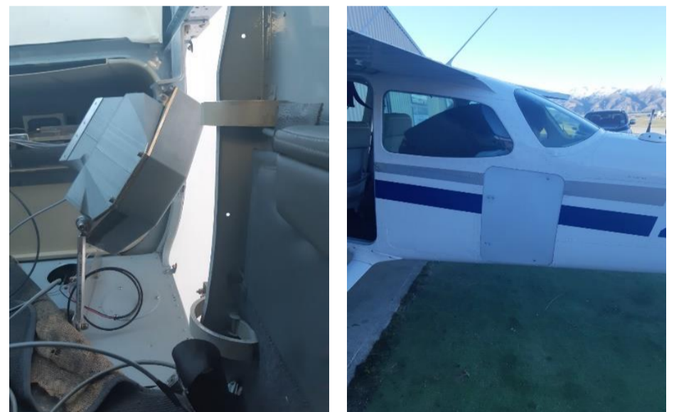
Figure 5: Left - SlimSAR L-and P-Band synthetic aperture radar (SAR). Right - Aircraft
